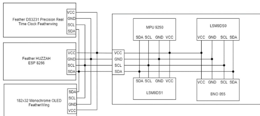
Fig. 4. Outline diagram of communication connections in the system
