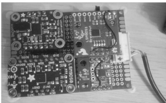
Fig. 5. Made gyroscope system with selected gyros
