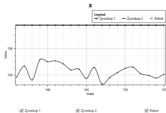
Fig. 13. Comparison of gyroscope reading results for the X coordinate
