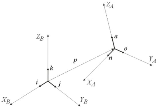
Fig. 1. Rotation matrix and orientation of system A axis in relation to system B
