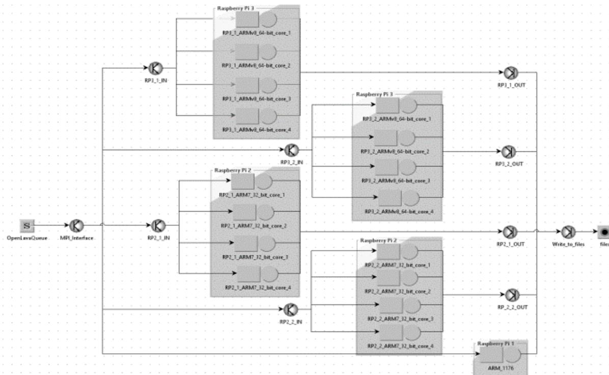
Fig. 1. Architecture of Raspberry Pi HPC cluster
